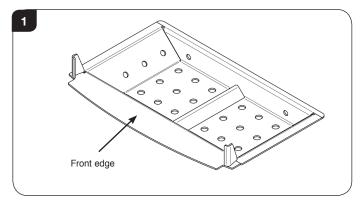
1.1 First remove the riddling mechanism from the appliance as detailed in the Installation and User instructions.
