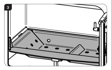
1.5 Fit the plug supplied into the hole where the riddling mechanism is normally located and secure with bolt and clamp (also supplied), see Diagram 4.
